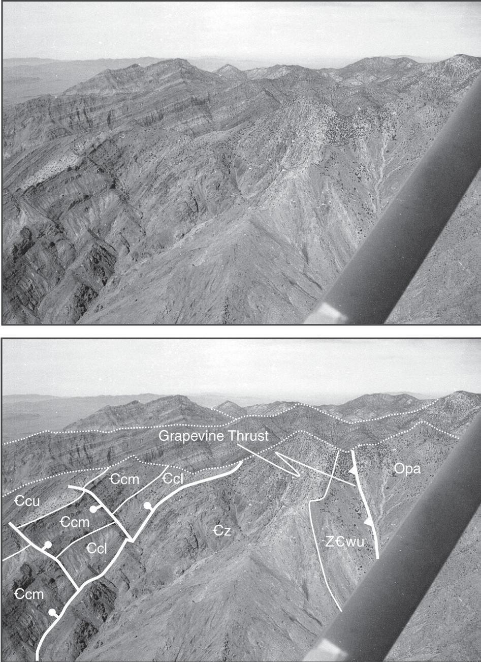
Figure 14. The Grapevine thrust in the central Grapevine Mountains, looking north toward Grapevine Peak. Note overturning of Grapevine thrust along the overturned limb of the Titus Canyon anticline. Area in this figure is in the left center of Figure 12. Unit abbreviations as on Plate 1. Dotted lines are ridge lines.
