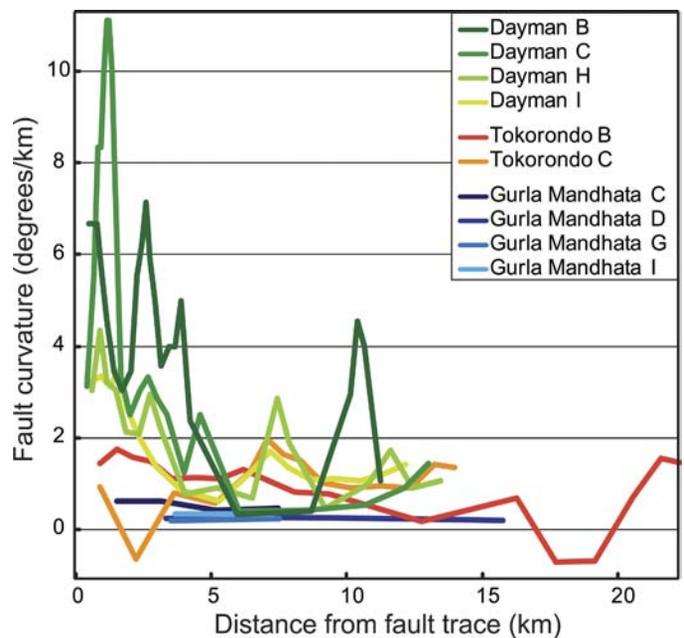
Figure 2. Fault curvature along selected displacement-parallel topographic profiles of three known or inferred detachment-fault footwalls. The spikes and troughs, especially apparent in the Dayman B cross section, result at least partly from differential erosion, where spikes represent subtle but developing ridges and troughs represent incipient stream valleys.
