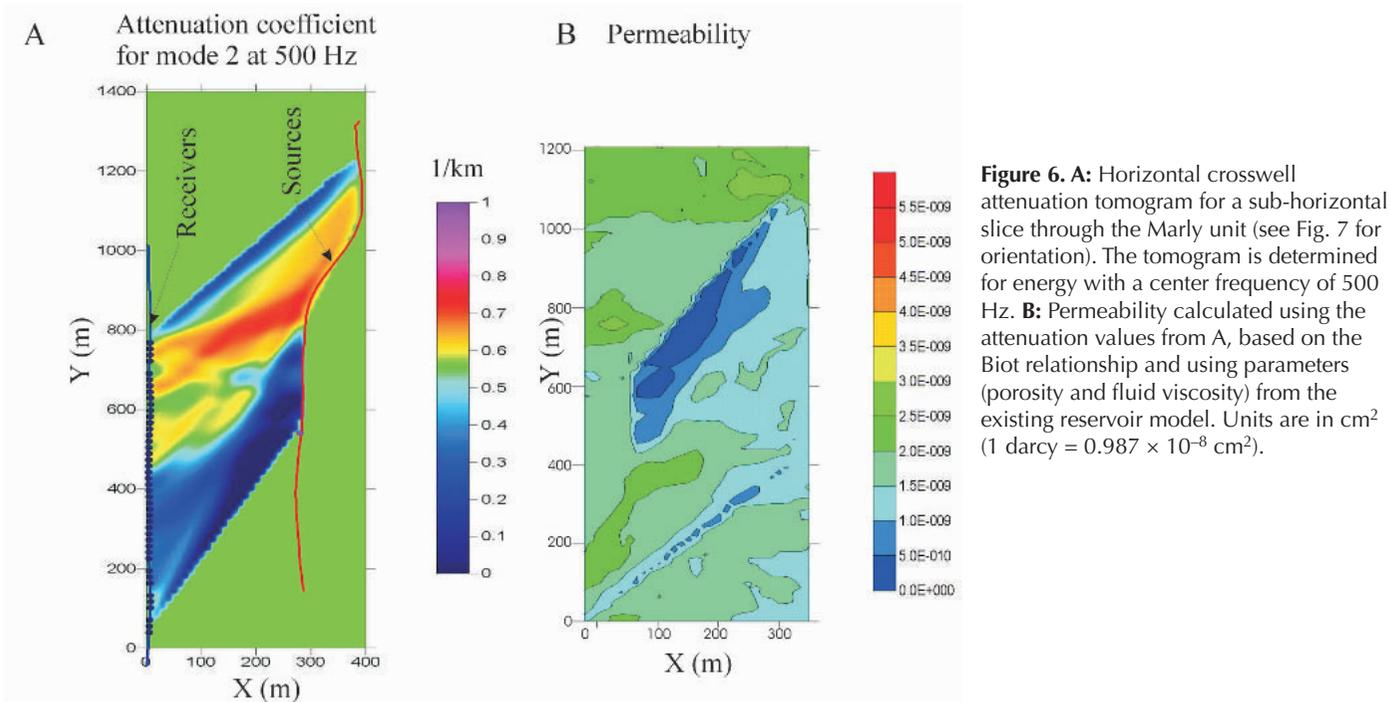
**Figure 6. A:** Horizontal crosswell attenuation tomogram for a sub-horizontal slice through the Marly unit (see Fig. 7 for orientation). The tomogram is determined for energy with a center frequency of 500 Hz. **B:** Permeability calculated using the attenuation values from A, based on the Biot relationship and using parameters (porosity and fluid viscosity) from the existing reservoir model. Units are in  $\text{cm}^2$  (1 darcy =  $0.987 \times 10^{-8} \text{ cm}^2$ ).
