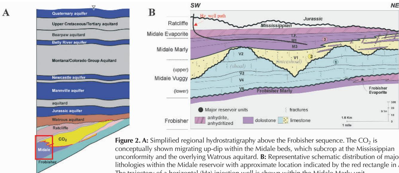
**Figure 2. A:** Simplified regional hydrostratigraphy above the Frobisher sequence. The CO<sub>2</sub> is conceptually shown migrating up-dip within the Midale beds, which subcrop at the Mississippian unconformity and the overlying Watrous aquitard. **B:** Representative schematic distribution of major lithologies within the Midale reservoir with approximate location indicated by the red rectangle in A. The trajectory of a horizontal (Hz) injection well is shown within the Midale Marly unit.
