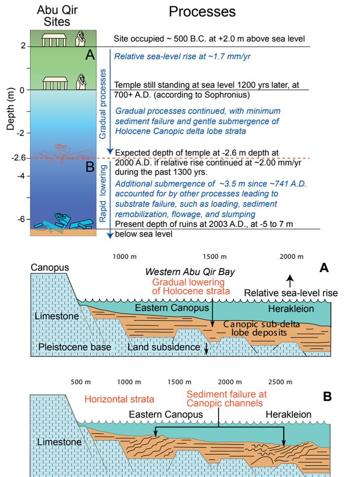
**Figure 7.** Interpretation of processes that submerged Herakleion and Eastern Canopus to depths of 5–7 m below sea level, from ca. 500 B.C. to the present. Processes involved: (A) gradual lowering of strata (as in Fig. 4A) and substrate failure (as in Fig. 4B). Discussion in text.
