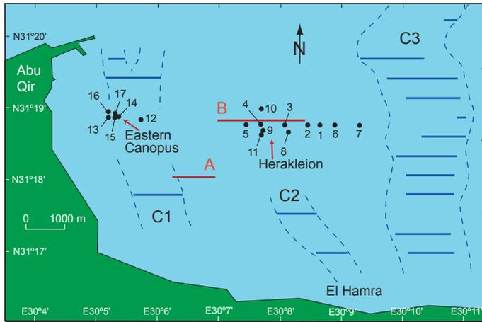
**Figure 2.** Western Abu Qir Bay, showing locations of Heracleion and Eastern Canopus and two selected high-resolution seismic profiles (red lines, shown in Fig. 4). Numbered dots show 17 vibracore sites. Three Canopic sublobe channels (C1, C2, C3) are revealed by seismic profiles (blue lines) and cores detailed in Stanley et al. (2004); these channels once extended >5 km north of the present coast. Depth and horizontal scale in meters.
