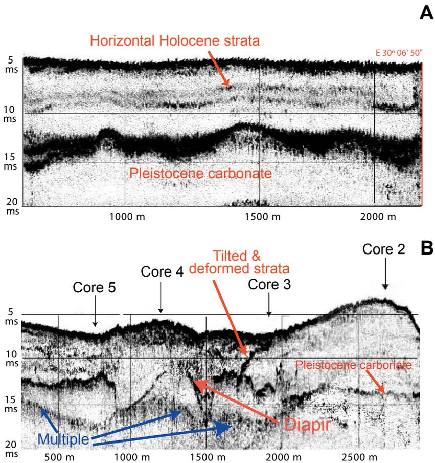
**Figure 4.** High-resolution profiles in Abu Qir Bay (location in Fig. 2) showing (A) Holocene horizontal strata above Pleistocene limestone base, between Herakleion and Eastern Canopus, and (B) tilted and deformed Holocene substrate directly under Herakleion ruins. Depth in milliseconds (10 ms = 7.5 m); horizontal scale at base of profiles in meters (vertical exaggeration ranges from 40 (in A) to 80 (in B).
