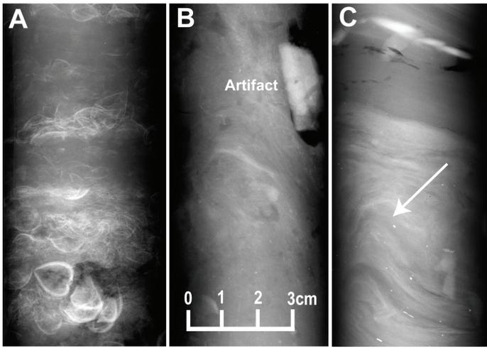
**Figure 6.** X-radiographs of split-core sections in study area (core sites in Fig. 2). **A:** Core 15 (depth ~110 cm from core top), showing typical delta wetland facies comprising bedded shell horizons in organic-rich silty mud matrix. **B:** Core 5 (depth ~13 cm from core top), with potsherd artifact in sediment-remobilized mud section. **C:** Core 9 (depth ~100 cm from core top), illustrating fluidized section with well-developed flame structure (arrow).
