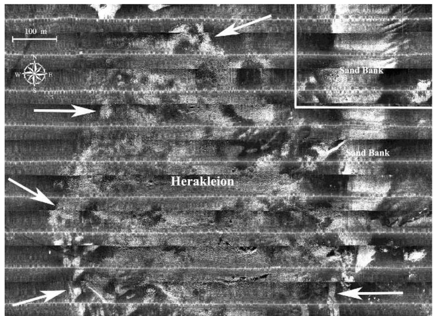
**Figure 3.** Side-scan sonar image partially shows the oval configuration of Heracleion ruins (arrows delineate general city limits) at water depths of 5–7 m. Diver exploration shows feathery patterns in upper right panel are tilted and uplifted mid-Holocene strata exposed on the bay floor. Each side-scan swath = 80 m.
