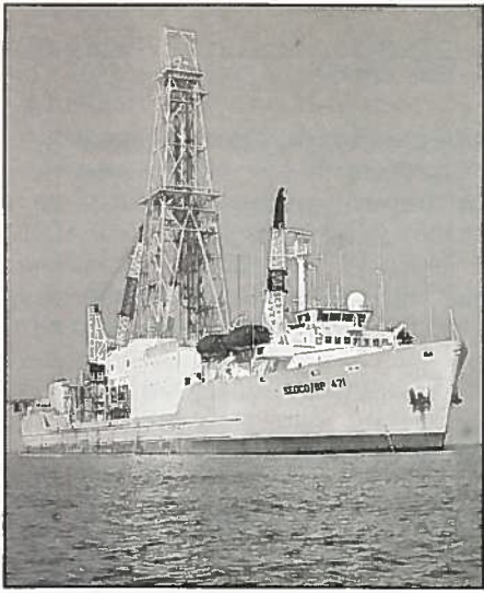
View of Joides Resolution (registered as SEDCO/ BP 471 ), the drilling ship of the Ocean Drilling Project. The ship dimensions are 143 m length, 21 m beam, 18,000 T displacement. The derrick is 62 m high; the ship carries 9150 m of drill string. The ship has 1115 sq m of laboratory space and accommodations for 68 crew and 51 scientific and technical party. The cruising speed is 11 knots, and the cruising range is 120 days.
