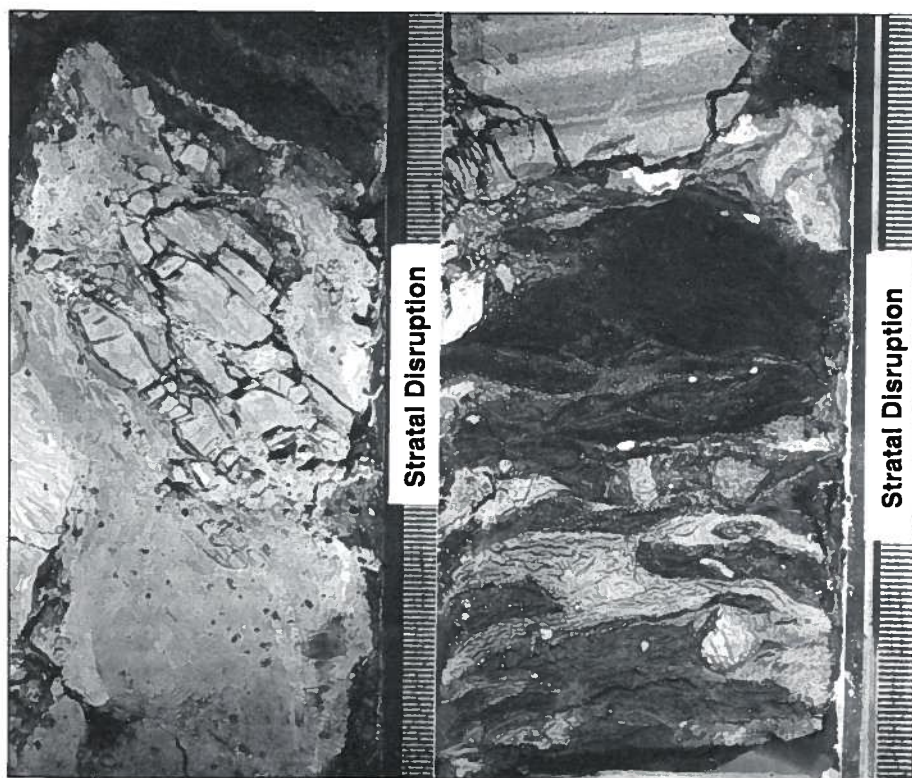
Figure 4. Stratal disruption developed cores sampled from 260 m subbottom from Site 674 of the northern Barbados Ridge (Brown and Behrmann, 1990). Stratal disruption developed adjacent to an out-of-sequence thrust (Fig. 5). Some of the horizontal banding in the core section to the right is due to drilling deformation, but geologic processes caused the dispersion of sandstone fragments. Scale to right of the core is in millimetres.
