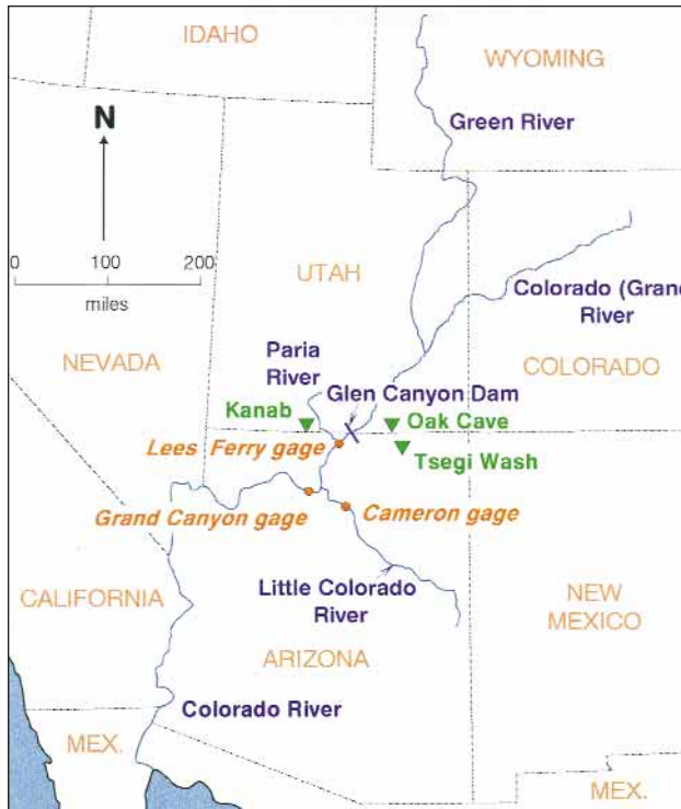
Figure 1. The only tributaries shown in this location map are the Paria and the Little Colorado Rivers, which are pertinent to this paper. Rivers are in blue; stream gages are in orange. The Lees Ferry gage measures the discharge from Glen Canyon Dam. The Cameron gage measures the discharge of the Little Colorado River, except for the relatively small flow from a spring near the confluence with the Colorado River. The Grand Canyon gage measures the combined discharges of the Colorado, Little Colorado, and Paria Rivers, plus the contribution of small tributary streams within the Grand Canyon, and minus seepage and evaporation losses. Oak Cave and Tsegi Wash, in green, are the location of Holocene deposits discussed in the text.
