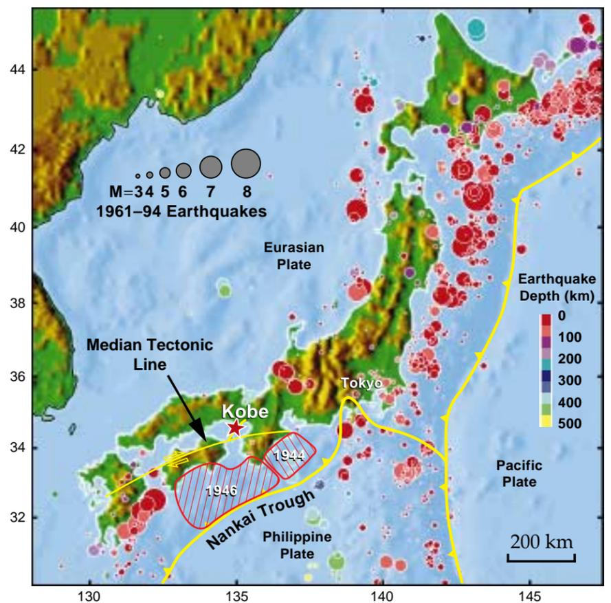
**Figure 3.** Japan, showing seismicity from 1961 to 1994, location of the 1995 Hanshin-Awaji earthquake, and projected rupture areas of largest historical earthquakes to shake Kobe, which were subduction-zone earthquakes in 1944 and 1946. (Figure prepared by Grant A. Marshall, U.S. Geological Survey.)
