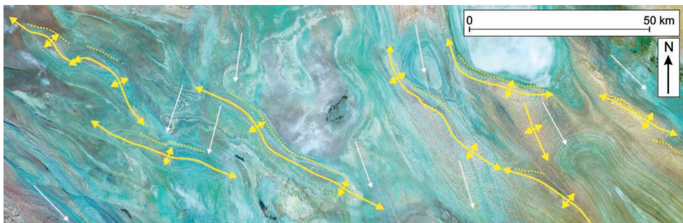
Figure 5. Landsat 7 image of the northwestern Qaidam basin (location shown on Fig. 2A). White arrows—prevailing wind direction during yardang development; yellow lines—axial traces of fault-propagation anticlines; yellow dotted lines—steeper forelimbs of anticlines (perpendicular to propagation direction).
